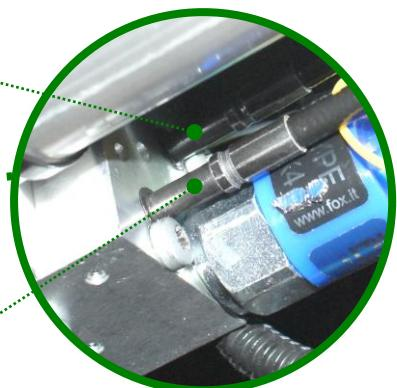
Note: Remove the protective plastic sleeves that are placed over the hydraulic nipples just before actual installation on the pump-unit, to avoid unnecessary dirt, or damage to the nipples.
